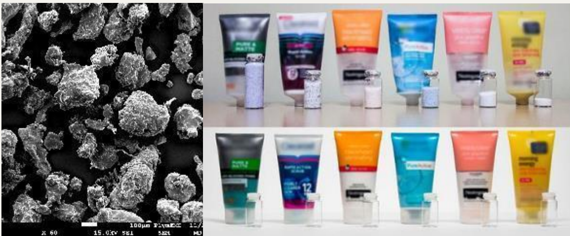
Figure 1. Left: Intentionally added microplastics (microbeads) extracted from a cosmetic product (60 times magnification); Top right: microbeads extracted from a range of cosmetics in 2015, shown in small jars in front of the product. Some of these products contain millions of these plastic particles. Bottom left: the same products had no such particles (empty jars) after UK legislation in 2018. Source: University of Plymouth
