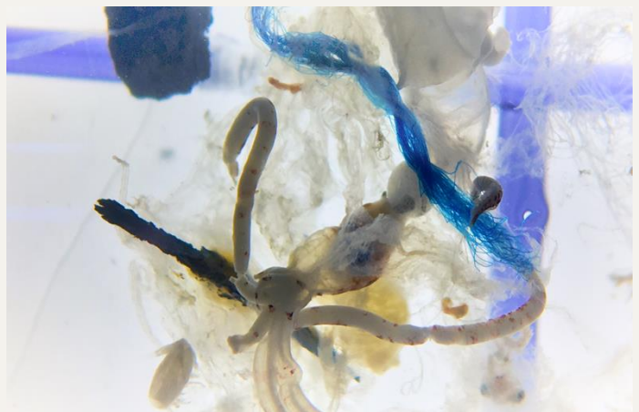
Figure 1. Microfibers mixed with natural debris from water sampled from the Pacific Ocean off the coast of Oregon (photo credit: Anna Bolm, Oregon State University). Polycarbonate filter imaged via Leica stereoscope at 20x magnification.
